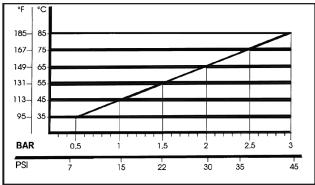
Naturally, if the application allows for feeding the pump with 45 psi (3 bar) even at low temperatures (for example: 115°F/45°C) the life of the wet end of the pump will be even longer.
